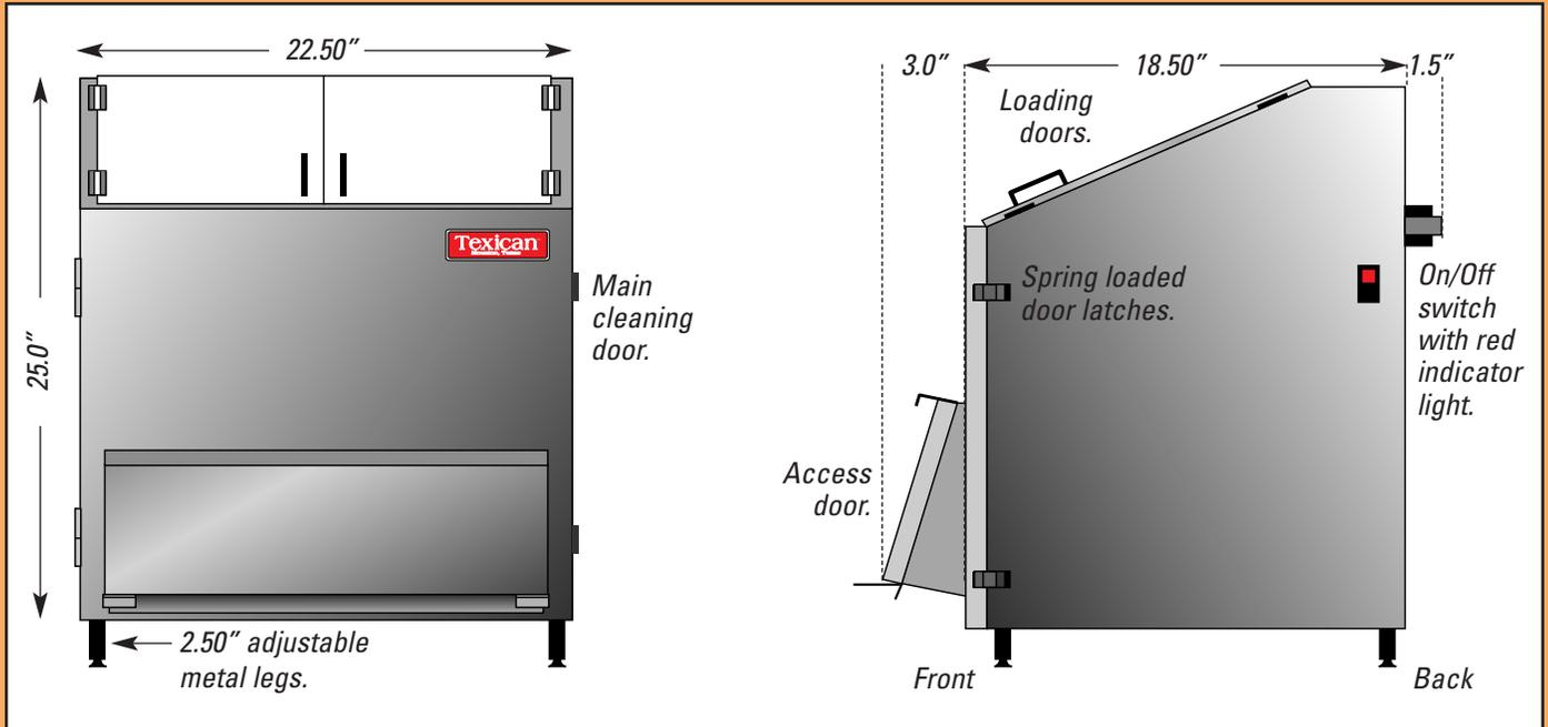
**Option: .250 thick anodized aluminum loading doors.**
