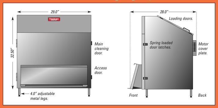
Option: .250 thick anodized aluminum loading doors.
