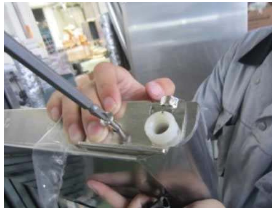
H. Assemble the door, then rotate it about 180 degrees. Assemble top hinge (right) with stopper plate in bottom hinge (left) position. (First, assemble top hinge (left); second, assemble bottom hinge (left) while doors are closed, insert hinge into door bushing (left) with lifting, rotate doors counter-clockwise, screw hinge in original positions.)
